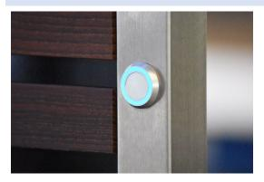
The MSK SLX snowmaschine visualize their operating status with a blink code on the piezo button or with text messages on the PLC in the control box. Additional data can be read from the PLC or individual settings can be made.
